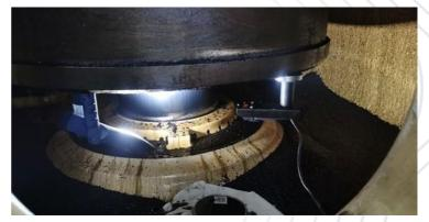
The stroke lenght and position of the piston is found by using laser.
