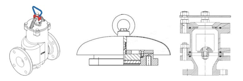
Due to the long vent pipes, it is vital that the high velocity pressure relief valves installed at the end of the vent line do not have any pressure surge above its opening setting, this is crucial to avoid any overpressure in the vent system. If the end of line high velocity pressure vacuum valve is installed, no further device needs to be installed for protecting the methanol tanks.
