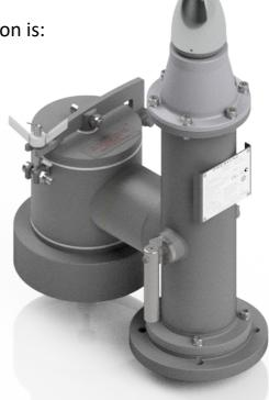
Due to the long vent pipes, it is vital that the high velocity pressure relief valves installed at the end of the vent line do not have any pressure surge above its opening setting, this is crucial to avoid any overpressure in the vent system. If the end of line high velocity pressure vacuum valve is installed, no further device needs to be installed for protecting the methanol tanks.
